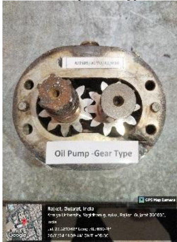
Oil Pump- Gear Type
