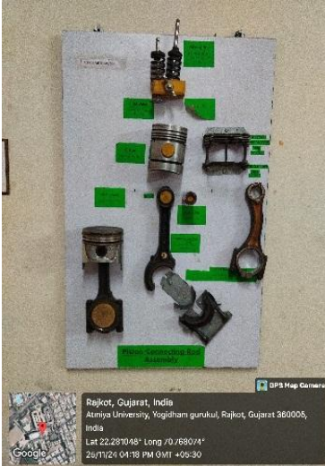
Piston Connecting Rod Assembly
