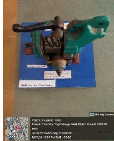
Steering Gear Box - Warm & Ballnut
