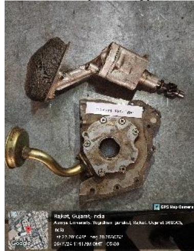
Oil Pump- Vane Type
