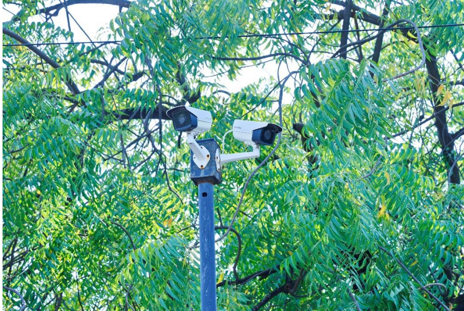
Motion & IR Sensor based energy saver camera
