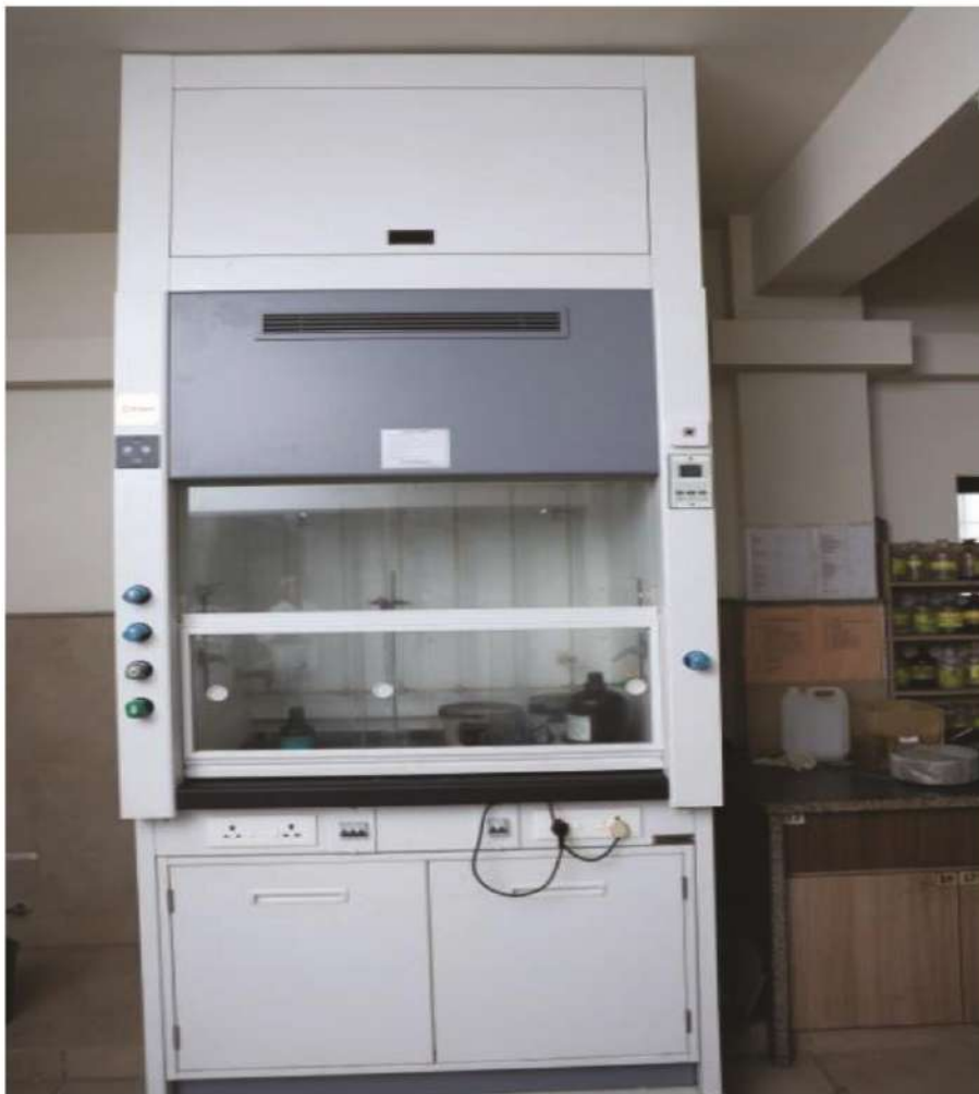
Fumehood at Chemistry Laboratory
