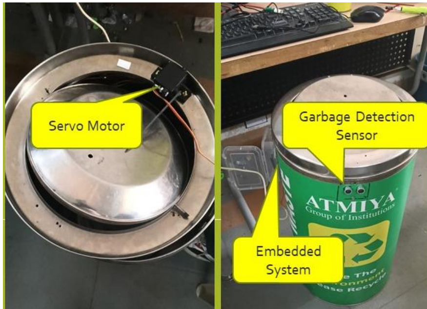
Technology Transferred Smart Dustbin installed at the University
