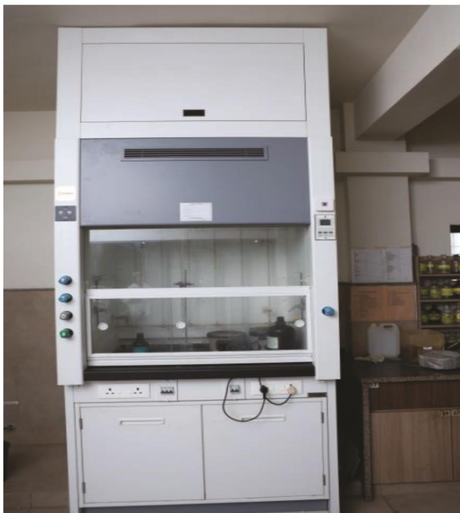
Fumehood at Chemistry Laboratory
