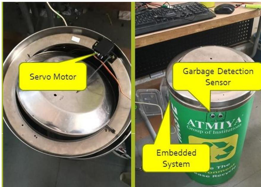
Technology Transferred Smart Dustbin installed at the University
