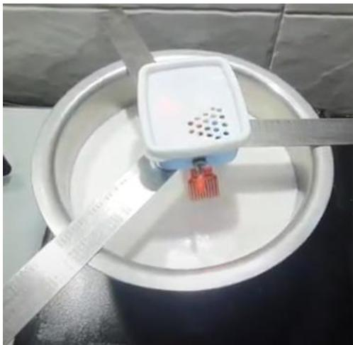
The device detects milk levels in a vessel using a water level sensor. It is positioned so that when boiling milk rises and touches the sensor, the sensor generates an analog signal. This signal is sent to an ATtiny85 microcontroller, which triggers a 9V piezoelectric buzzer. The buzzer alerts the user to turn off the stove, serving as an alarm.
